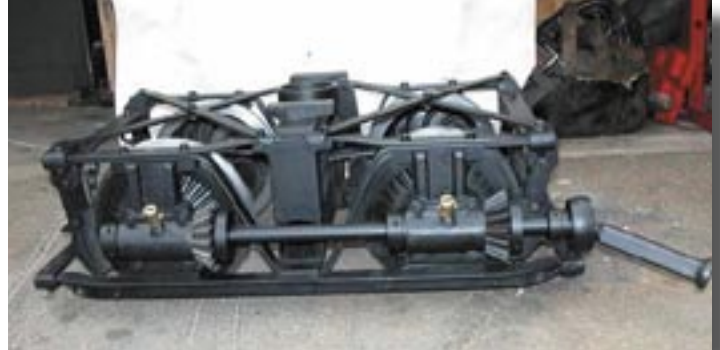
One of two rebuilt Shay trucks.
