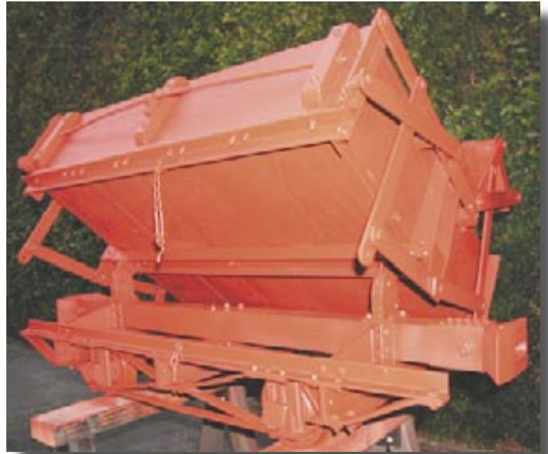
Newly restored side dump car.
